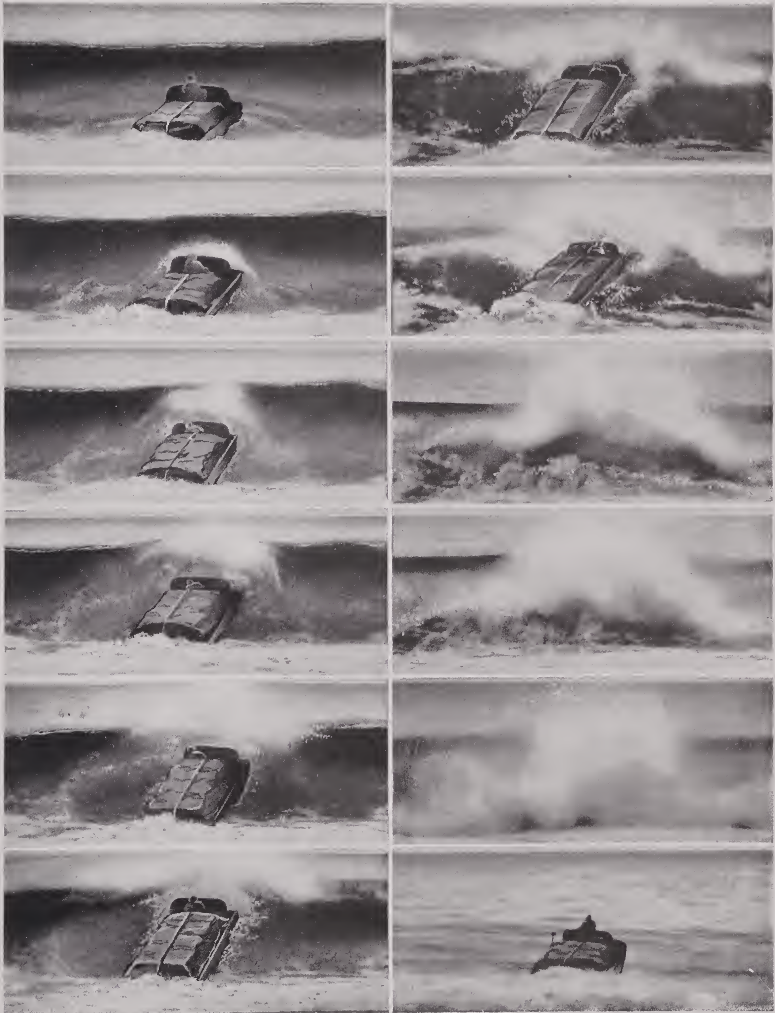
FIGURE 52. Series of photographs of laden DUKW penetrating 15-foot comber on steep-to beach at Monterey Bay, California, showing very rapid rise of bow due to shape and buoyancy of bow sections. Last picture shows course unaltered. Amount of water taken aboard is ejected by pumps in about 1 minute.
